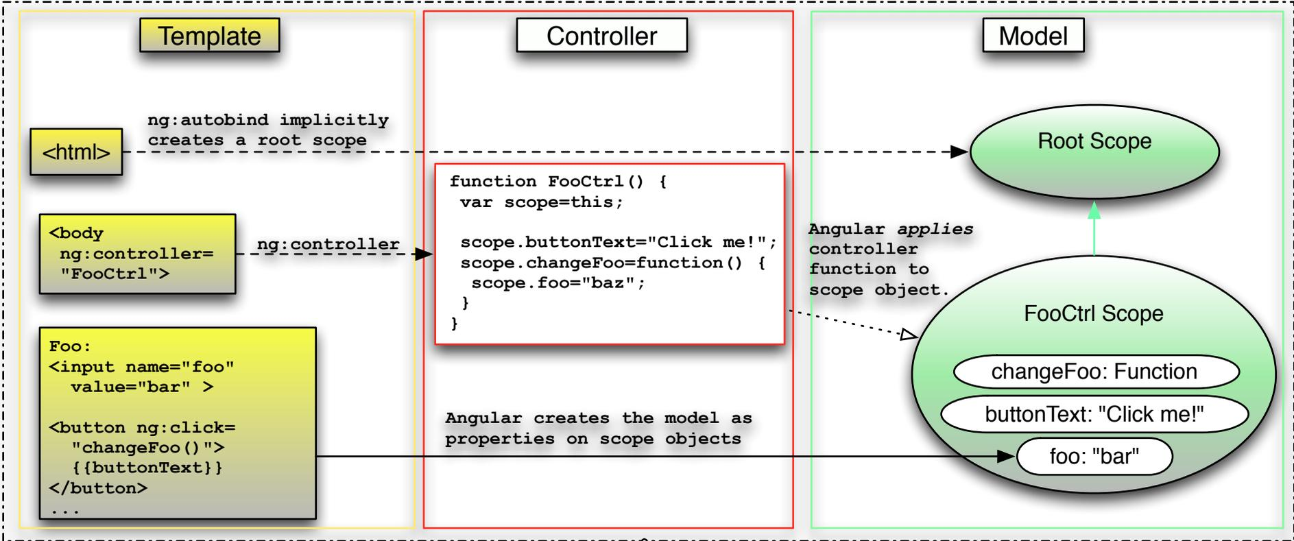
To generate the View, angular gathers information from the Template; applies Controller functions to associated Scope objects; links Model properties to the associated Scope objects; then generates a transformed DOM, which is rendered in the browser.
