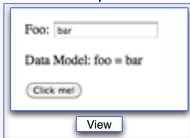
Angular sets up two-way data-binding between the value of the property "foo" in the FooCtrl scope, and the input text box in the View.
